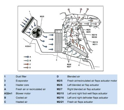
130. As a vehicle's HVAC system cools air, condensation forms on a component called an evaporator (labeled "3" in the diagram above). In a non-defective system, this condensation is evaporated through the activation of a fan and airflow over the evaporator.
