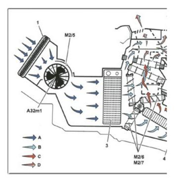
63. As a vehicle's HVAC system cools air, condensation forms on a component called an evaporator (labeled "3" in the diagram above). In a non-defective system, this condensation is evaporated through the activation of a fan and airflow over the evaporator.
